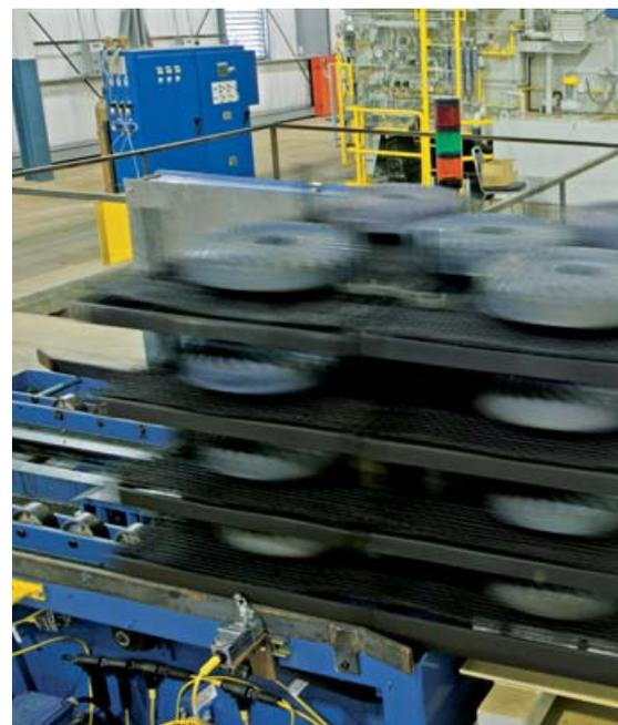
the furnace to receive the load at a specific time. A fully automated cart, powered by MOVITRANS®, travels to the right spot to handle the entire process from dispatch of material all the way to the furnace and back. MOVITRANS® does not need any festooning or overhanging cabling. It is a compact system routed in the floor that is at the heart of a solution for a multi-faceted challenge. Adams states that MOVITRANS® represents enormous labor savings. "The heat-treating
