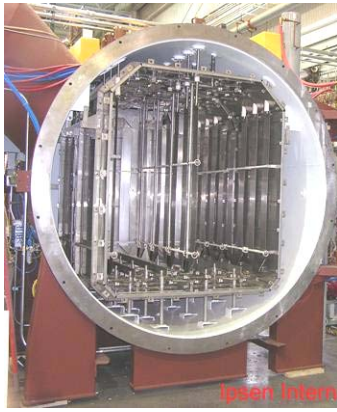
Figure 18 Vacuum Aluminum Brazing Furnace with Center Heating Element
