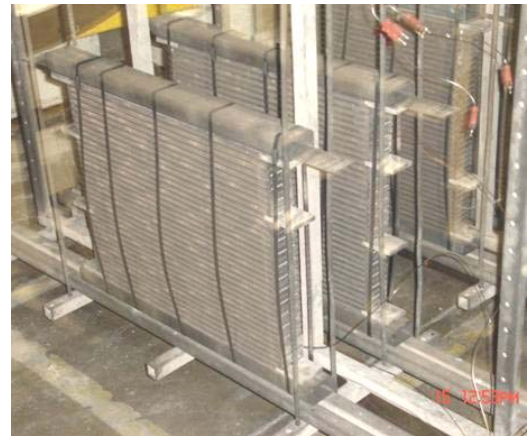
Figure 14 Band Type Fixturing (Photo courtesy of API Tech)
