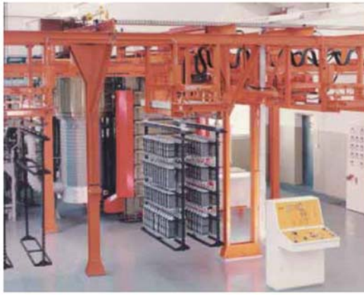
Figure 6 Semi-continuous Furnace Load Carrier and Conveyor System
